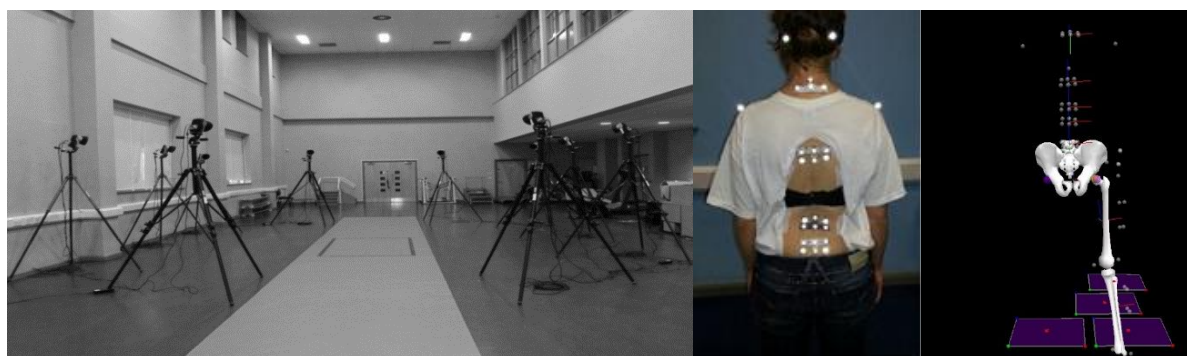
FIGURE 2 (LEFT) The AHRu movement lab (Brook Building, UCLan) (CENTRE) Adapted t-shirt for marker placement and collection of spinal data. (RIGHT) Static model in software (Visual3D, CMotion, MD, (USA)).
